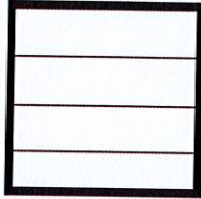
Lid Concrete lid in 4 parts Lid thickness 3 inches Reinforcing rod 6 mm at 4 inch distance
