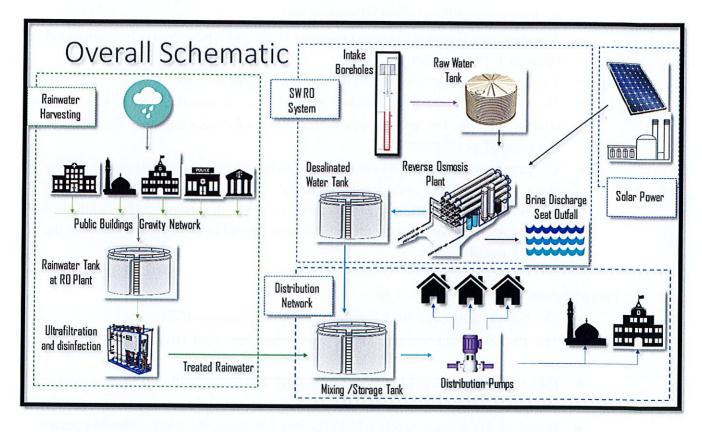
The Water Supply System design should be based on IWRM systems which include the following components (Where one of these components are available in the island the system should be designed to incorporate the other components)
