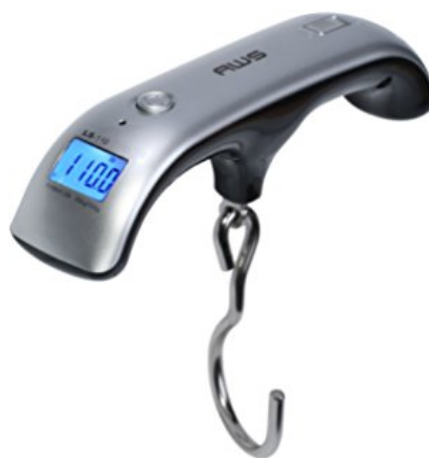
Figure 20: Electronic hook scale used to measure the mass of waste during the survey
