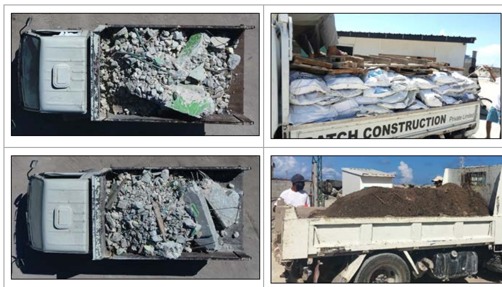
Figure 37: (a) Aerial view of a 2T truck containing concrete waste (b) Truck containing sand and rocks in polypropylene woven sacks with wooden pellets on top (c) Aerial view of a 2T truck containing concrete waste (d) Truck containing soil.
