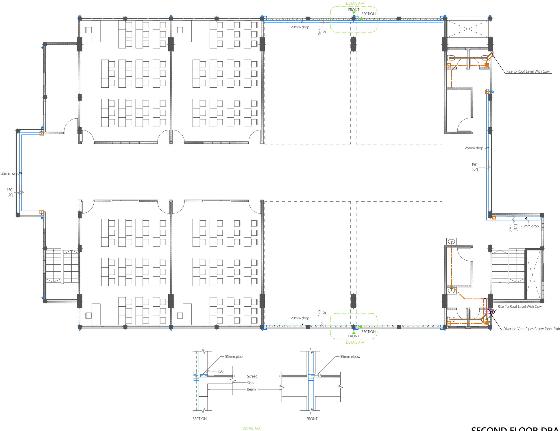
SECOND FLOOR DRAINAGE LAYOUT 1:150
