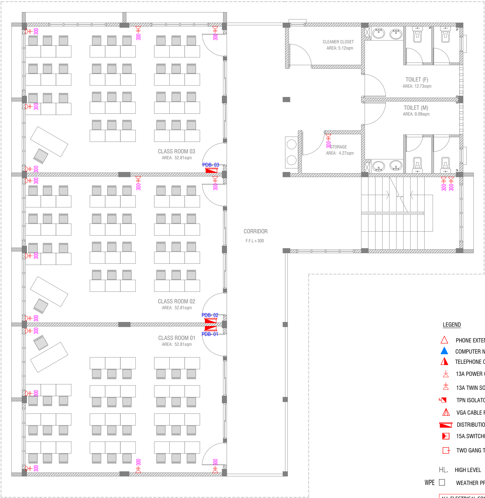
FIRST - THIRD FLOOR POWER LAYOUT SCALE 1:100
