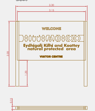
Sawed tropical wood pillar (Teak, Iroko, Cerejato or similar), from 14x14 to 20x20 cm per section and up to 4 meters long, structural quality MEG, resistant class C-18, protection of the wood with penetration class P2, worked in a workshop.
