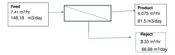
A treatment plant consisting Dual media filtration, Activated Carbon filtration, Anti scalant dosing, Micro filtration and RO membranes separation system and CIP system is proposed with necessary pumps and storage facilities.
