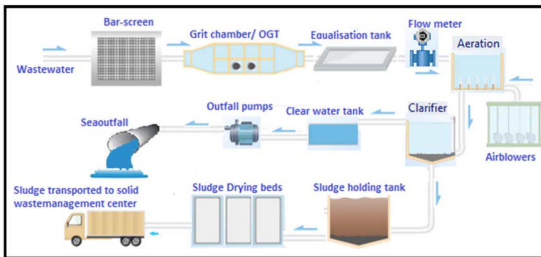
Figure 1: Activated Sludge process diagram
