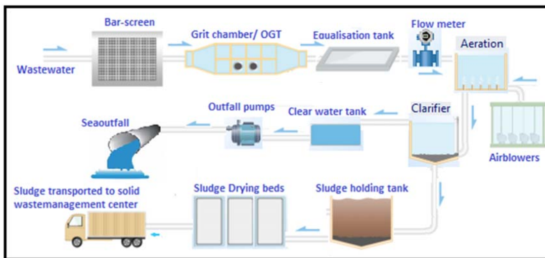
Figure 1: Activated Sludge process diagram
